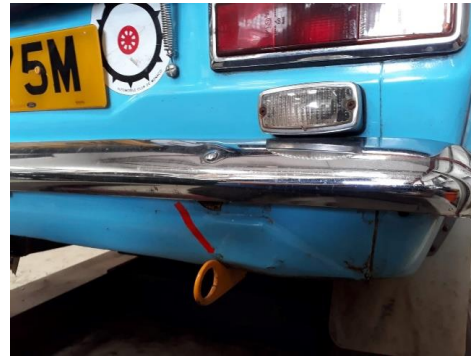
Rear using arrow sticker and painted orange
